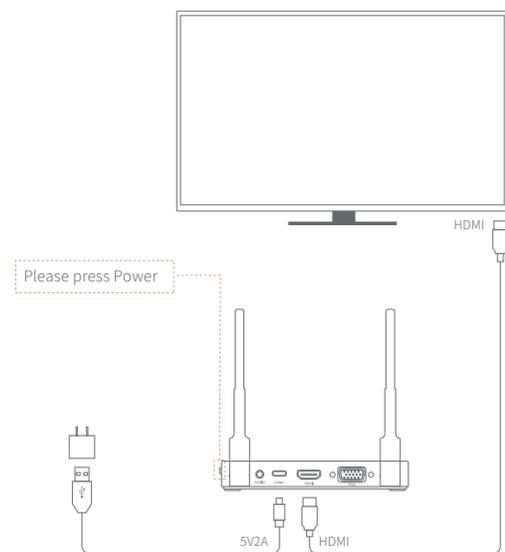
1. Insert the HDMI cable in the accessory into the HDMI port of the receiver (RX), and connect the other end HDMI cable input port of the large screen display terminal (TV or other equipment).
