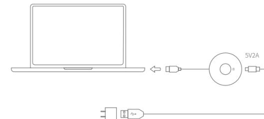
1. Plug the transmitter's power supply into the adapter or USB power port (voltage: 5V/2A), and then the transmitter's HDMI interface.
