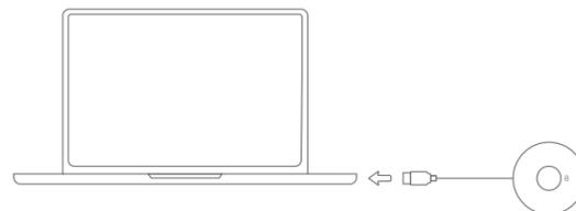
Insert the transmitter (TX) HDMI cable into the computer HDMI output port. After waiting for ten seconds, you can project the laptop screen to the big screen and complete the projection. (Please ensure that the computer is fully charged)
