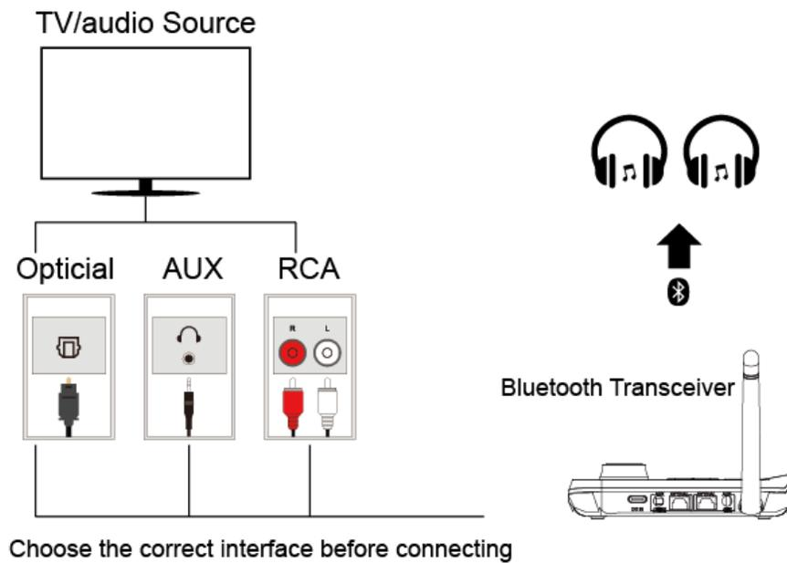
**Fig 3: Set up Bluetooth transceiver as Bluetooth transmitter**
