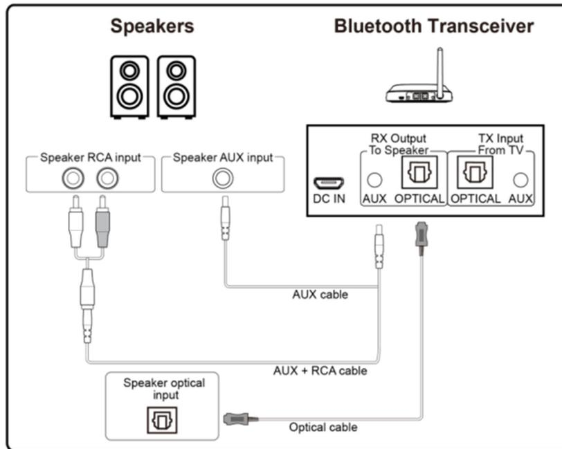
**Fig 1: Set up Bluetooth transceiver as Bluetooth Receiver**
