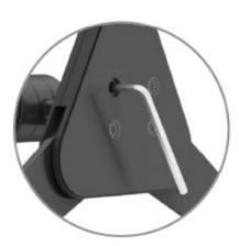
To change the tension on the ball joint, remove the four silicone plugs on the front of the mount to reveal the Allen head screws. Use an Allen wrench to tighten or loosen the screws, as desired.
