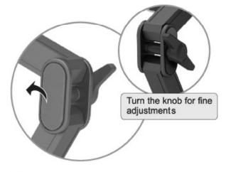
Remove the silicone pad on the mounting arm joint to reveal the arm-joint tension screws. Turn the knob for fine adjustments.
