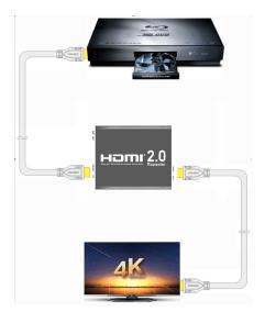
1. Use the HDMI cable to connect the HDMI output interface of the DVD/BD to the HDMI IN interface of the repeater.
