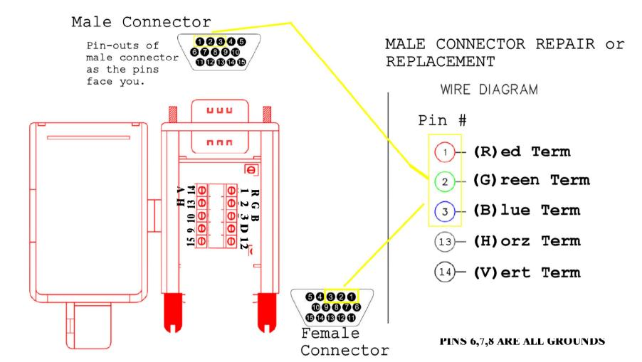
Locate the wire attached to PIN #1 of your existing VGA connector. You will attach this wire to the "R" connector on the replacement block. Do the same for #2, and #3. Pin 4 is not used. Pin 13 goes to "H", and pin 14 goes to "V".
